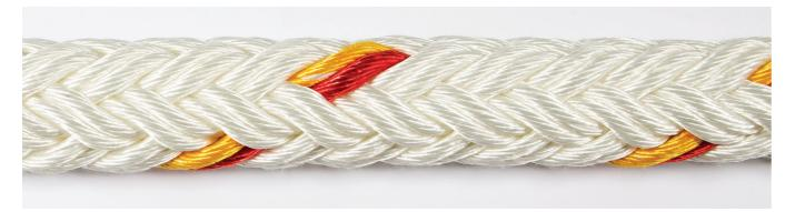
**Nika-Flex 12/24-Strand Ropes** are mixed Polyolefin & Polyester ropes. High tenacity Polyester fibers cover Nika-Steel® fibers through an engineered twisting process. The selected twist factor & fiber tensioning make the Nika-Flex yarns stronger and more abrasion resistant than conventional mixed yarns. All of the strands are composed of mixed Nika-Flex yarns and the resulting Polyester percentage is 50% - 50% w/w though the whole strand's cross-section.
