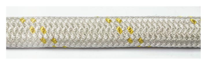
NIKA-Double Braided 100% Polyester Ropes are 100% Polyester ropes constructed by braiding a 32/64 strand sheath (or jacket) over a braided core.
