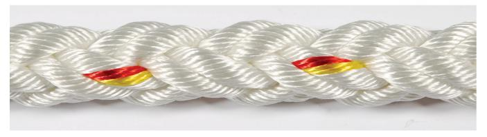
**Nika-Flex 8-Strand (4x2) Ropes** are mixed Polyolefin & Polyester ropes. High tenacity Polyester fibers cover NIKA-Steel® fibers through an engineered twisting process. The selected twist factor & fiber tensioning make the NIKA-Flex yarns stronger and more abrasion resistant than conventional mixed yarns. All of the strands are composed of mixed NIKA-Flex yarns and the resulting Polyester percentage is 50% - 50% w/w though the whole strand's cross-section.
